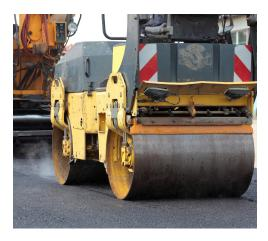
onboard display and computer reporting system. By integrating all components, IC rollers can accelerate project delivery as well as improve quality. IC rollers also collect enough data to display continuous records of the number of roller passes, material stiffness measurement values, and precise location of the roller.
